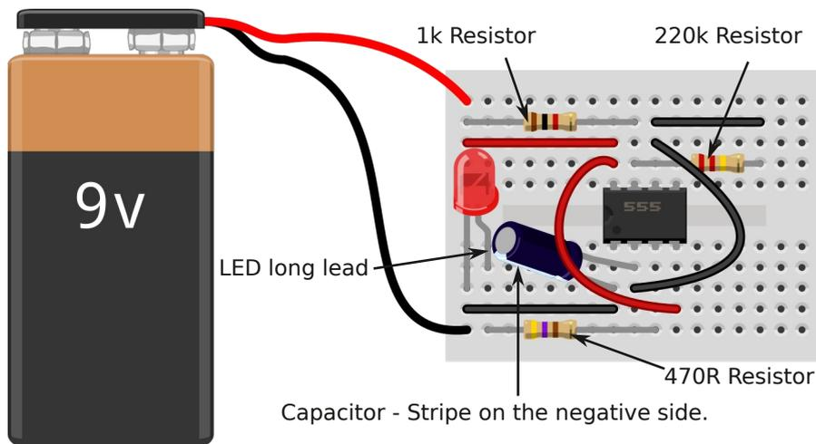
If everything has been assembled correctly you should see the LED flash at around 3Hz or 3 times per second. Troubleshooting: If the led does not start to flash straight away, disconnect the battery immediately. The cause of any failure will, almost certainly be due to getting components in the wrong position. Check that the polarised components are the right way round and that all leads are pushed fully into the breadboard.
